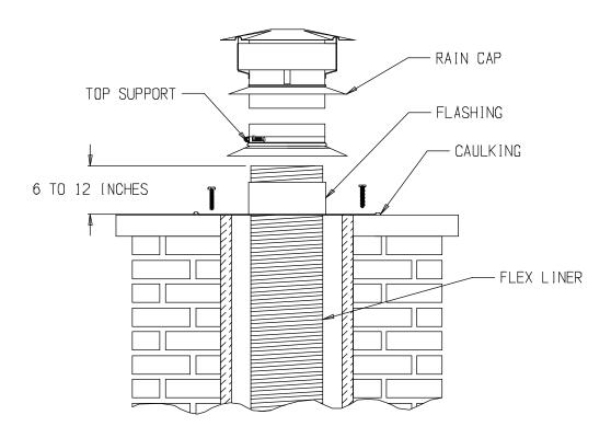
9. Slide Top Support over liner down to the top of the flashing collar allowing about a 1" overlap on the flashing collar. Trim the liner level to top of Support using a knife or hacksaw. Next, insert Rain Cap into the liner. Tighten up on gear clamp supplied on Top Support crimping liner onto the Rain Cap base allowing it to overlap the flashing collar preventing any rain from getting between flashing collar and liner.
